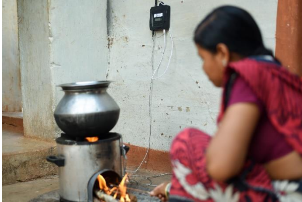
Figure 1: Improved cookstove equipped with a temperature sensor for remote monitoring.
